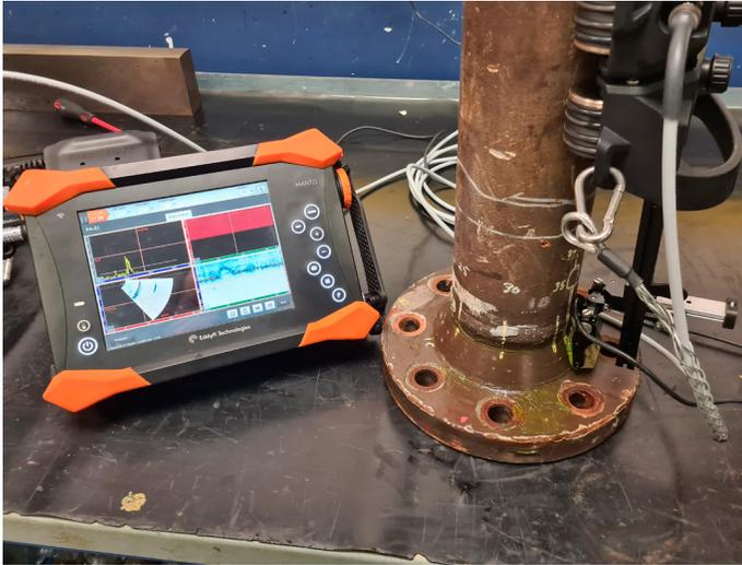
Figure 1: Flange face corrosion assessment with LYNCS™ and Mantis.
