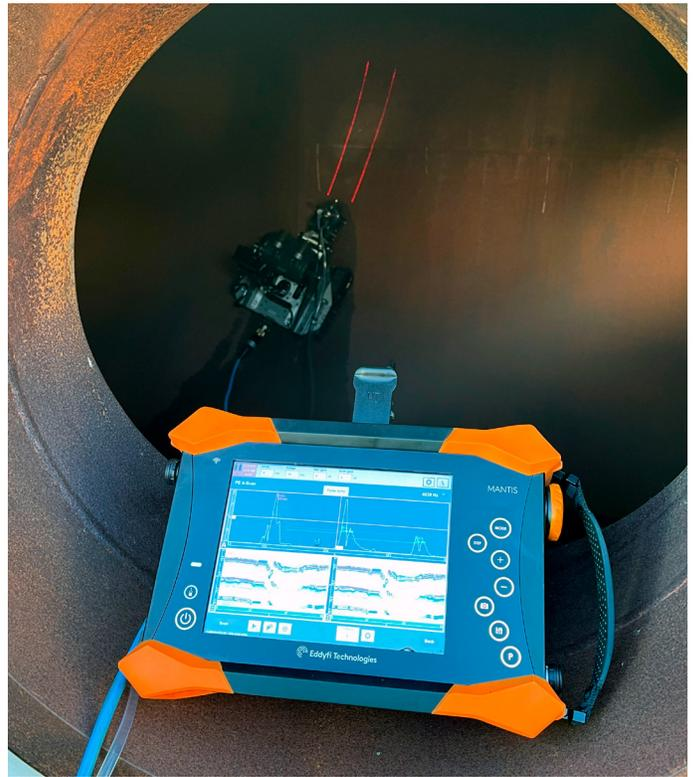
Figure 3: Mantis and VersaTrax™ for remote inspection.
