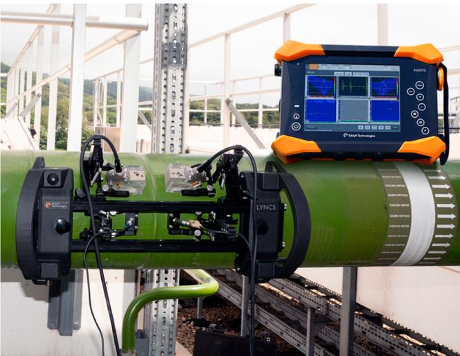
Figure 6: LYNCS scanner with Mantis for pipe inspection.
